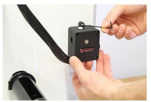
Insert the remaining 2 x M3 screws and tighten down.
