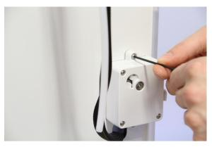
Unscrew the 2 x M3 screws that hold the original geared Ultimaker feeder into place.
