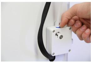
• Remove the collet clip, which locks the bowden tube into place.
