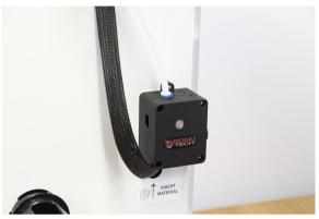
• Add the blue collet clip to lock the the bowden tube into place.
