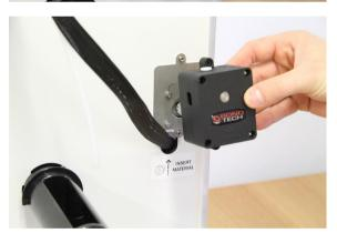
Place the Bondtech feeder assembly against the rear back plate.
